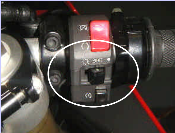
(old) manual switch
